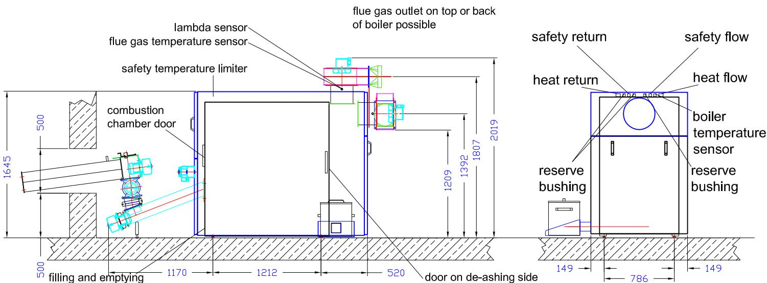
The boiler should be accessible from three sides. The discharging system should not cross the heating room.
