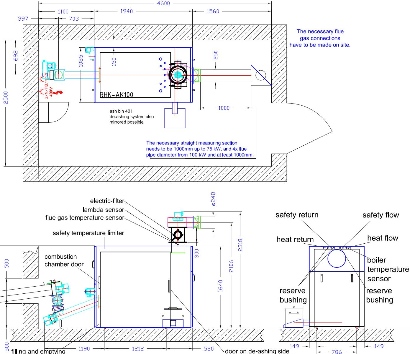
The boiler should be accessible from three sides. The discharging system should not cross the heating room. Room height and position of the particle separator(s)\* should be discussed with the Heizomat team. Connecting points for the necessary potential equalization on the boiler see supplementary sheets "Connection of the Heizomat boiler system to the main potential equalization of a building" \*.
