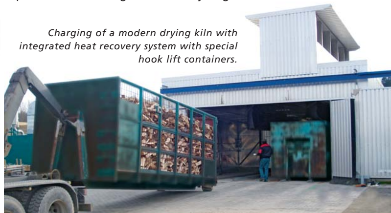
Hook lift container with air-permeable side walls for firewood drying.
