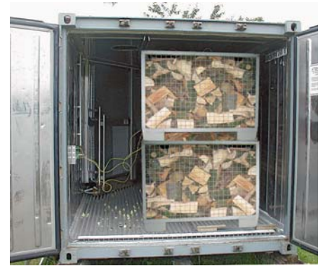
Skeleton boxes with 1 m 3 of firewood each in a small drying kiln (container solution).
